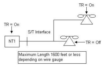
Fig. 6: Terminating Resistor Settings for Farthest Teleset
